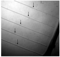
Figure 1: Drying channels (from top to bottom, 60, 80, 100, 120 and 140 µm in width). Arrows show the menisci.
