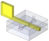
Figure 1: Sliding wall principle.
