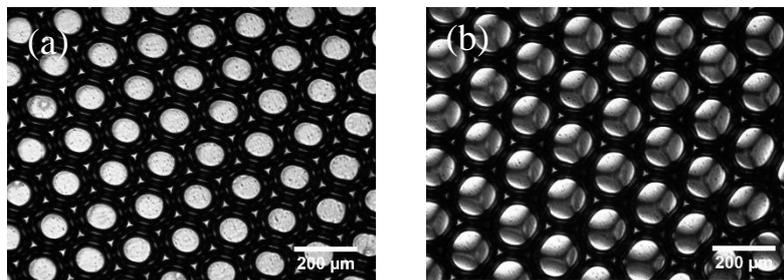
*Figure 1: Model foams generated by microfluidics. (a) Monodisperse bubble monolayer – (b) Monodisperse bubble bilayer.*
