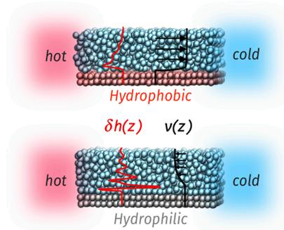
FIGURE 1 : Illustration of the thermo-osmosis flow
