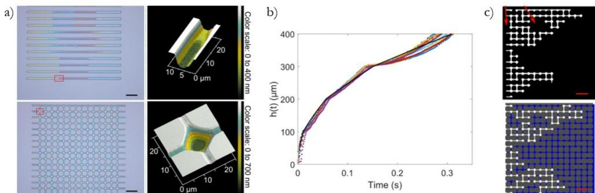
Figure 1: a) Picture after grayscale laser lithography and AFM image after etching. Top: varying depth nanochannels and zoom on a step. Bottom: pore network and zoom on a pore. b) Experimental (colored dots) and theoretical (black line) imbibition kinetics in a four steps nanochannel. c) Comparison between experiment (top) and pore network simulation (bottom) during the drainage of a 2.5D nanopore network. Red arrows point liquid cluster. Scale bar represents 50  $\mu\text{m}$ .
