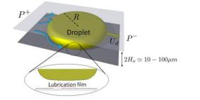
Fig.1 Squeezed droplet in a Hele-Shaw cell
