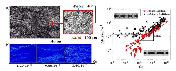
**Figure. 1.** a) Photo of a foam transport in a porous medium. b) Maps of different preferential paths.
