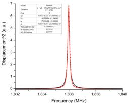
Figure 2: Mechanical Characterization in vacuum: the Lorentzian fit of the first mode peak. A Q factor of about 10.000 has been measured.
