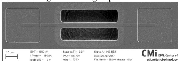
Figure 1: Microbeam with nanoslit channel (length 80  $\mu\text{m}$ , width 5  $\mu\text{m}$ , height 50 nm)
