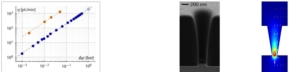
Figure 1: Measured flow rate through calibrated capillaries (left), SEM picture of a nanopore (center) and theoretical velocity field in low Reynolds regime (right).
