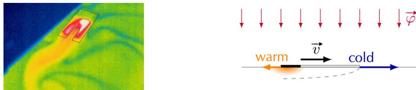
Figure 1: Infra-red view of a sun boat at a water/air interface (left) and schematic of the propulsion mechanism (right)
